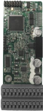
Resolver PG card EC-PG504-00
