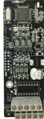
24V simplified incremental PG card EC-PG507-24
