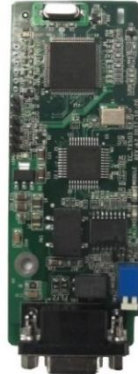
PROFIBUS-DP communication card EC-TX503D
