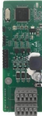
Simplified incremental PG card EC-PG507-12
