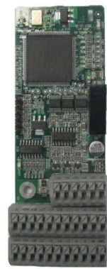
UVW incremental PG card EC-PG503-05
