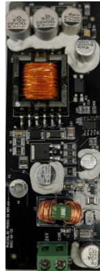
24V power supply expansion card EC-PS501-24
